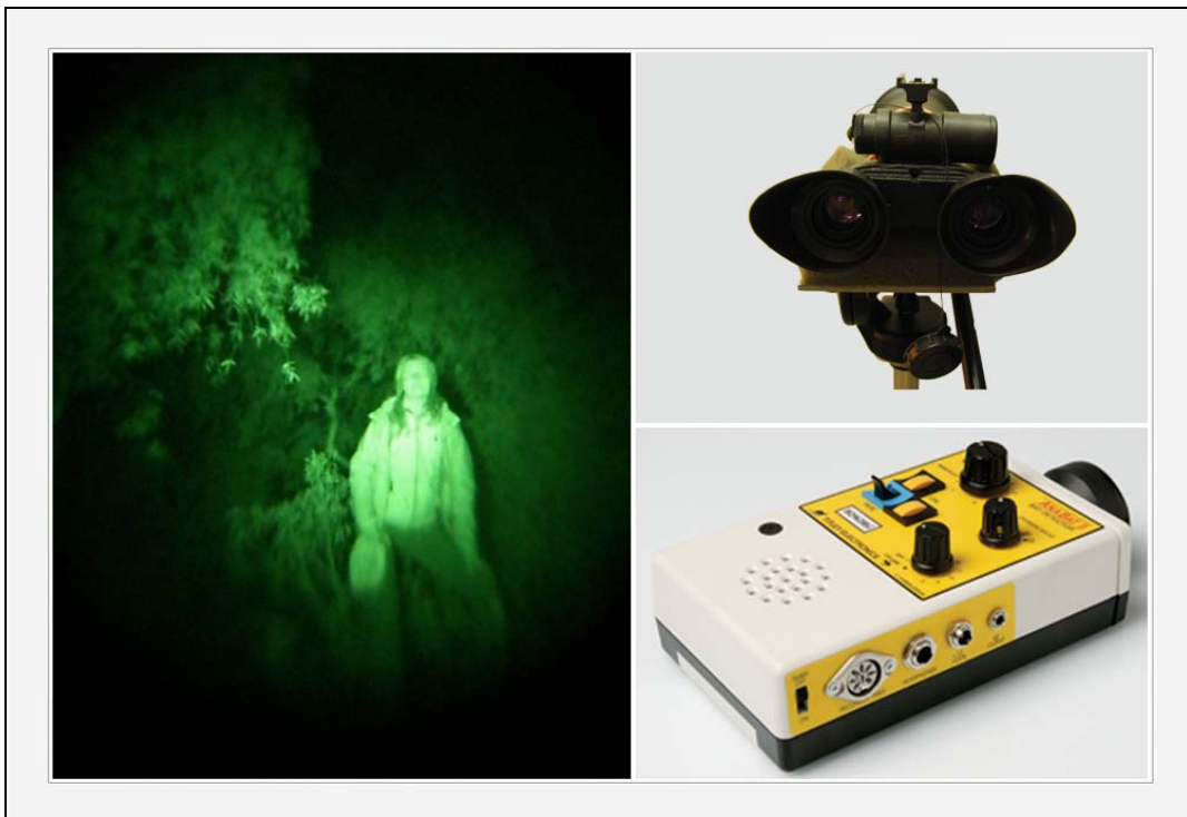
Fig. 7.1. Night-vision attained (left) with a generation-2 night vision device and an external infrared light focused on the part of the image that appears brightest. Note: image is unfocused as it was taken without camera adapter. A night-vision device mounted on a tripod (top right) and a bat detector (bottom right).
